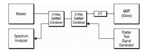
Figure 3-1. Conducted Test Setup for DFS
