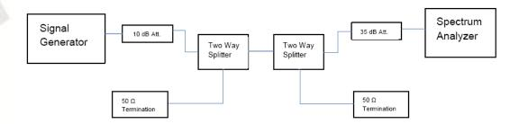
Figure 3-2 Test Setup for Conducted Measurement Radar Verification
