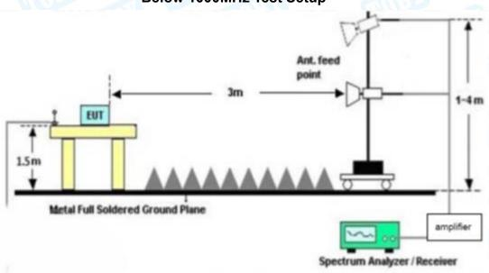
**Above 1GHz Test Setup**
