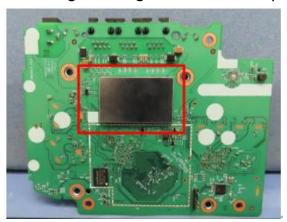
3. Adding gasket on the heatsink board
