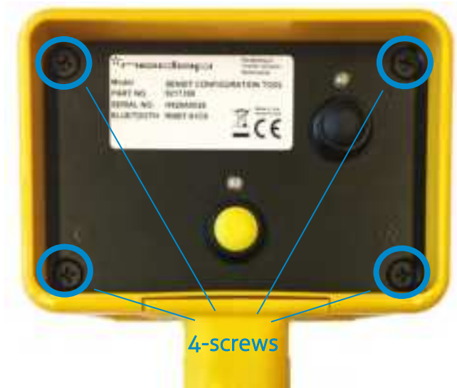
Figure 18: Configuration tool remove screws to open housing
