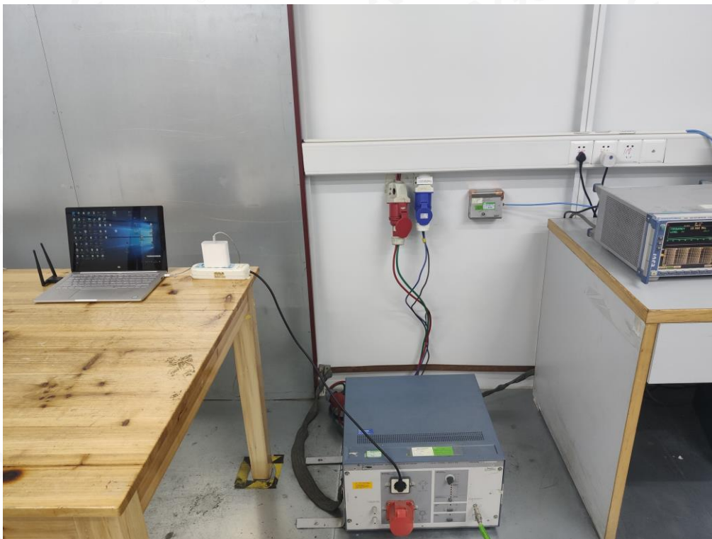
FCC RADIATED EMISSION TEST SETUP BELOW 1GHZ
