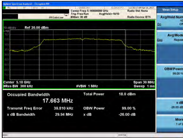
(802.11a) -26dB&99% Bandwidth plot on channel 40
