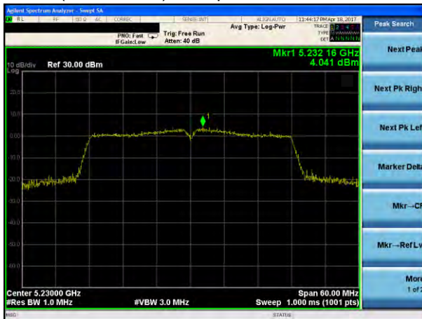
(802.11ac40) PSD plot on channel 46
