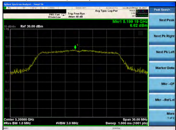
(802.11ac20) PSD plot on channel 40
