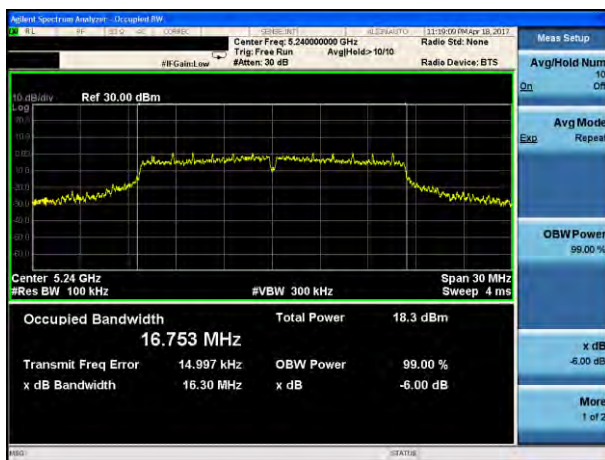
(802.11a) -6dB Bandwidth plot on channel 48
