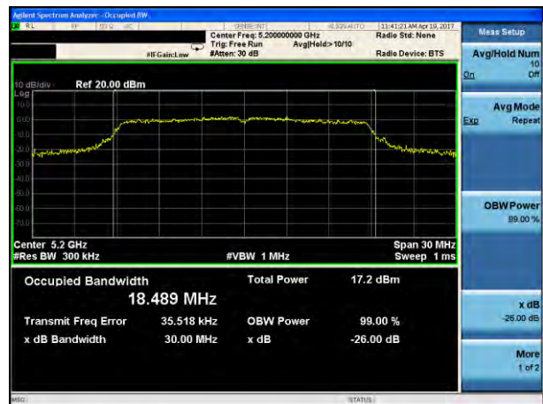
(802.11ac20) -26dB&99% Bandwidth plot on channel 48
