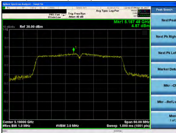
(802.11ac40) PSD plot on channel 38
