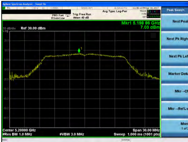
(802.11a) PSD plot on channel 40
