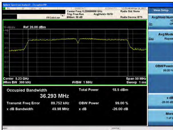
(802.11ac40) -26dB&99% Bandwidth plot on channel 46
