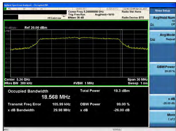
(802.11ac20) -26dB&99% Bandwidth plot on channel 48
