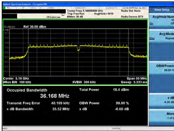
(802.11ac40) -6dB Bandwidth plot on channel 46
