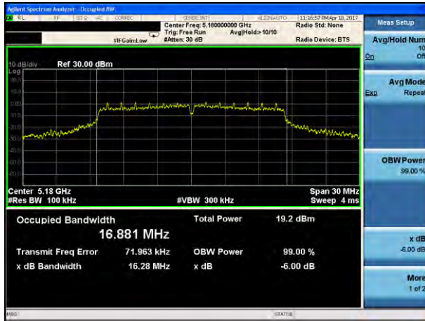
(802.11a) -6dB Bandwidth plot on channel 40
