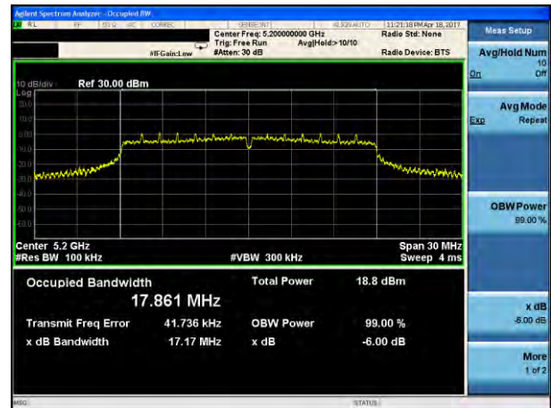
(802.11ac20) -6dB Bandwidth plot on channel 48
