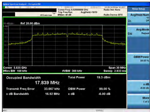
(802.11ac20) -6dB Bandwidth plot on channel 165
