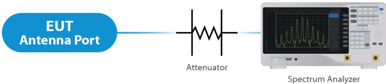
Figure 2: Direct Connect at the Antenna Port Test
