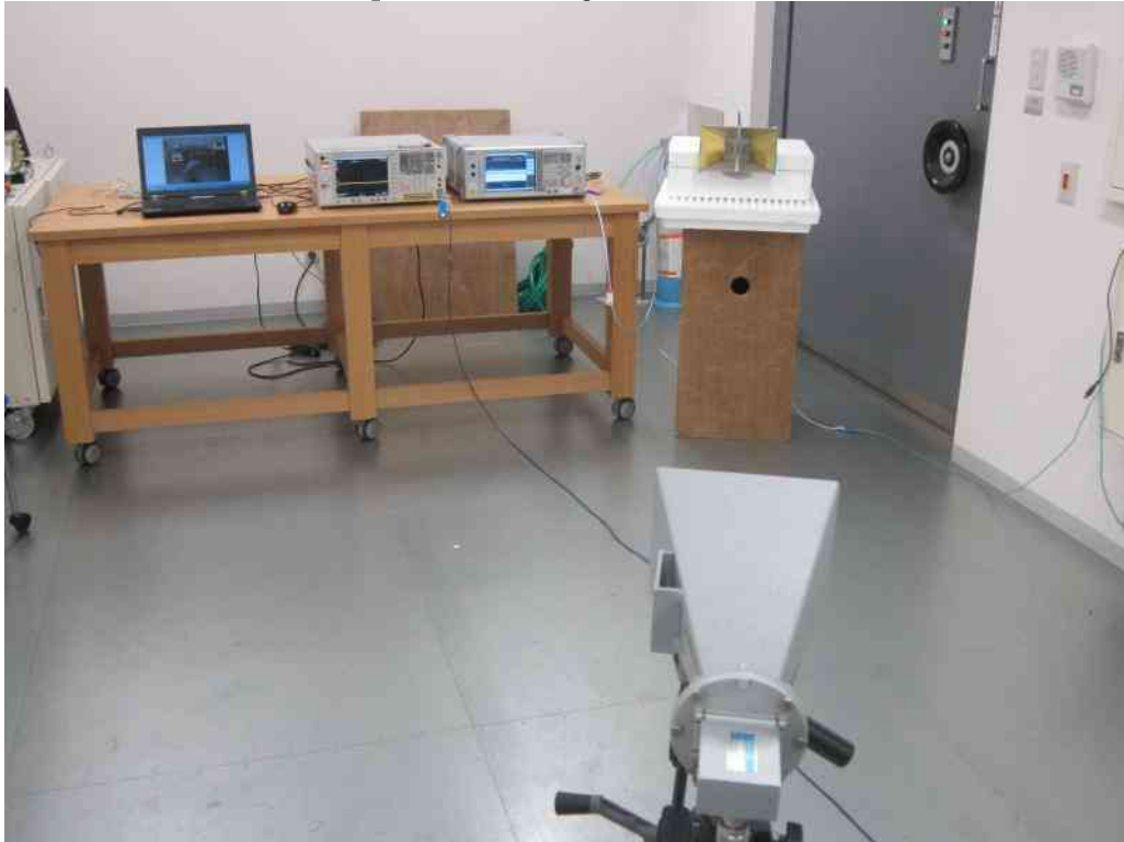
Test Setup for Generating the Radar Waveform
