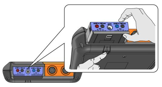
⇒ Now the MT 77 is instered in the module slot of the MT-HV.
