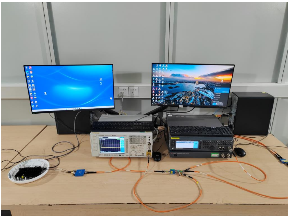
Description: DFS Test Setup
