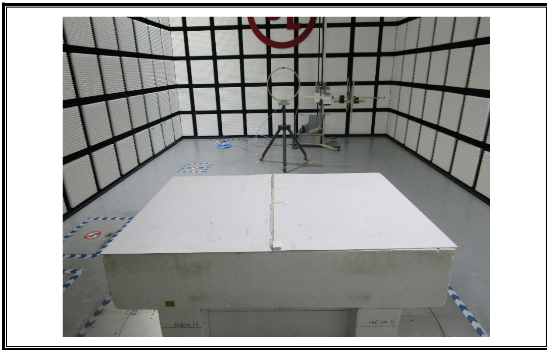
RADIATED RF MEASUREMENT SETUP (Below 30MHz)
