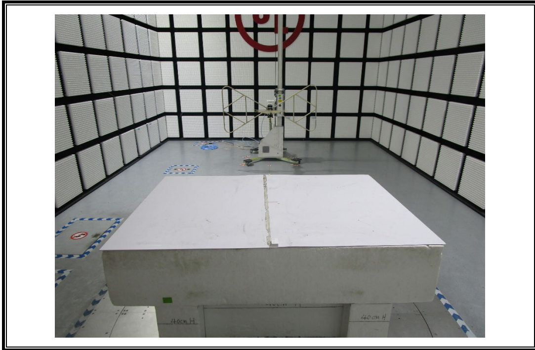
RADIATED RF MEASUREMENT SETUP (30MHz ~ 1 GHz)
