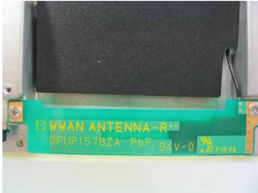
EVDO Main TX/RX Antenna
