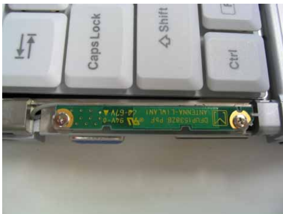
WLAN AUX TX/RX Antenna
