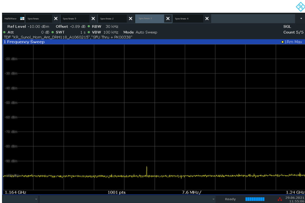
Plot 7-34. Radiated Spurious Pre-Scan 1164 - 1240 MHz - CH.9 - ANT 2 – GPS band
