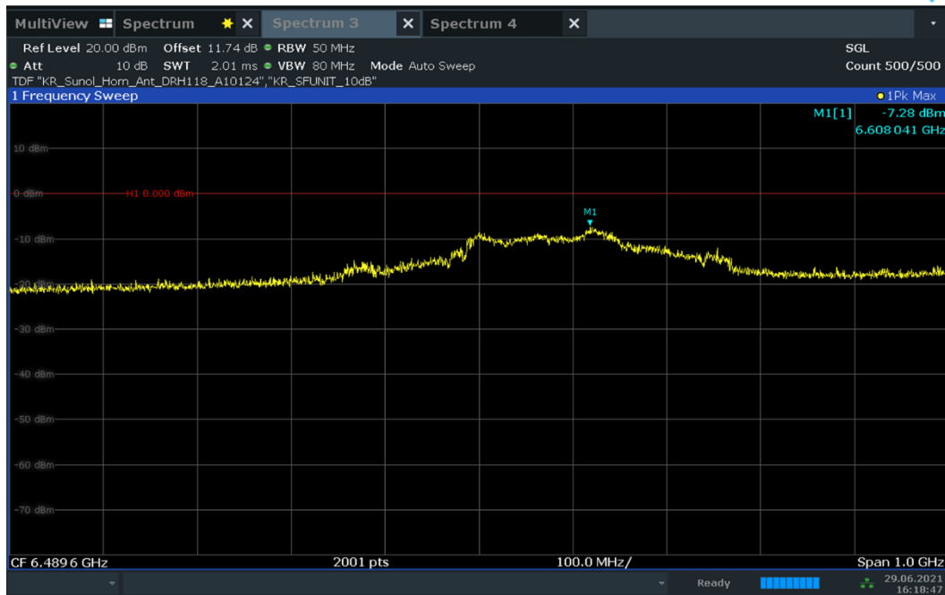
Plot 7-11. UWB Peak Power Measurement - ANT 2 - CH.5 – HPRF
