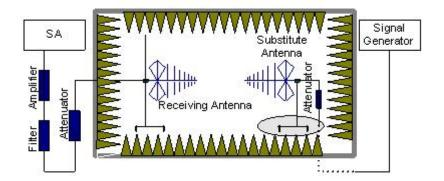
In the chamber, a substitution antenna for the frequency band of interest is placed at the reference point of the chamber. An RF Signal source for the frequency band of interest is connected to the substitution antenna with a cable that has been constructed to not interfere with the radiation pattern of the antenna. A power ( $P_{Mea}$ ) is applied to the input of the substitution antenna and adjusts the level of the signal generator output until the value of the
