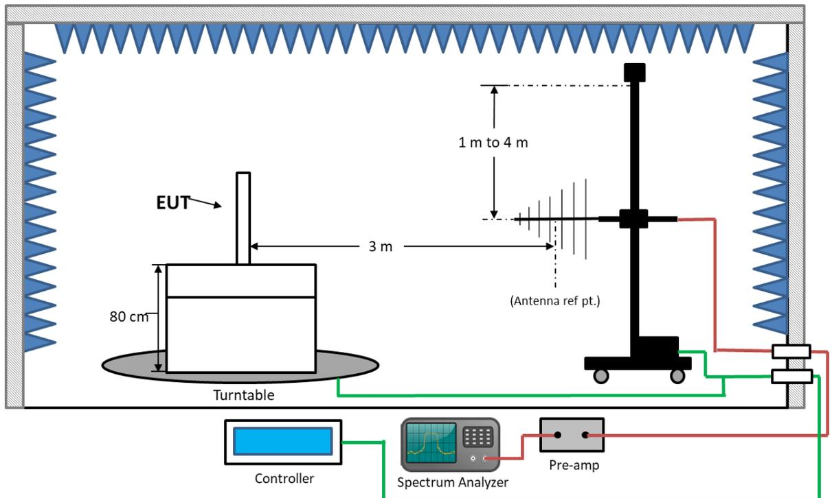
**Figure 1. EUT Test Configuration – Radiated Emissions**
