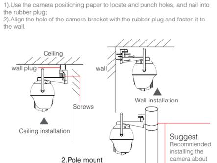
This product supports three installation methods: ceiling, wall and pole.
