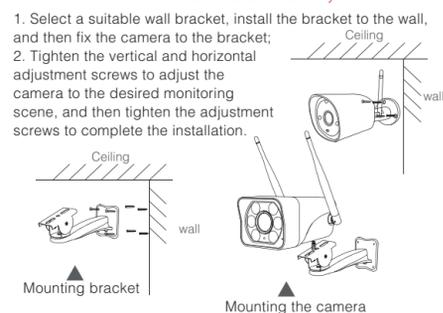
1. Select a suitable wall bracket, install the bracket to the wall, and then fix the camera to the bracket;
