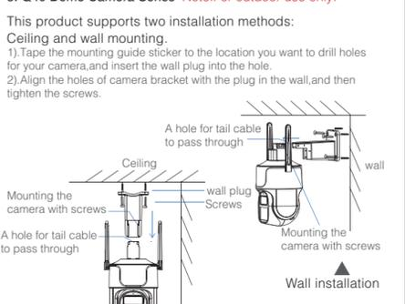
1).Use the camera positioning paper to locate and punch holes, and nail into the rubber plug;
