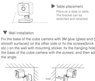
Fix the base of the cube camera with 3M glue (glass and other smooth surfaces) on the other side or fix the screws (brick wall, etc.) on the wall with mounting sticker, fix the hanging hole of the base of the cube camera with the screws, and then adjust the angle.
