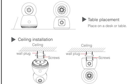
1. Insert the expansion plug into the ceiling and fix the bracketbase to the ceiling with screws;
