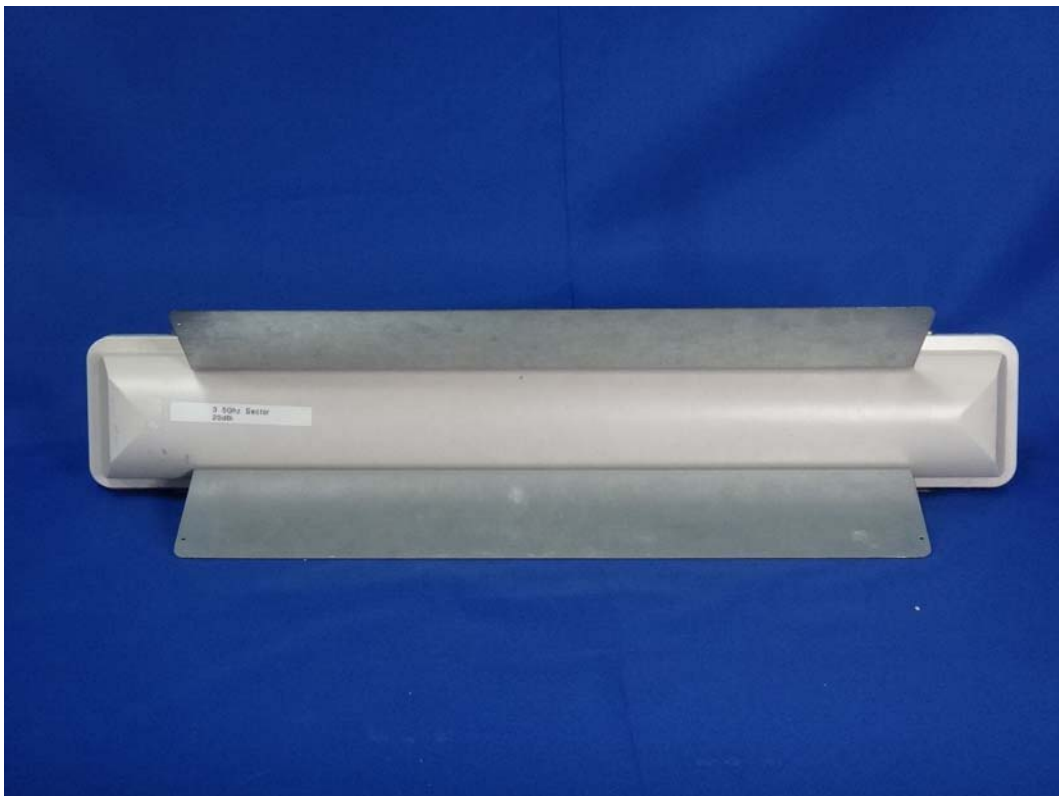
(12) EUT Photo (Sector Antenna)
