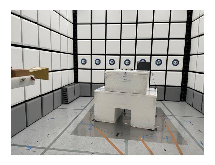
**Radiated Emissions Test Setup (Front)**
