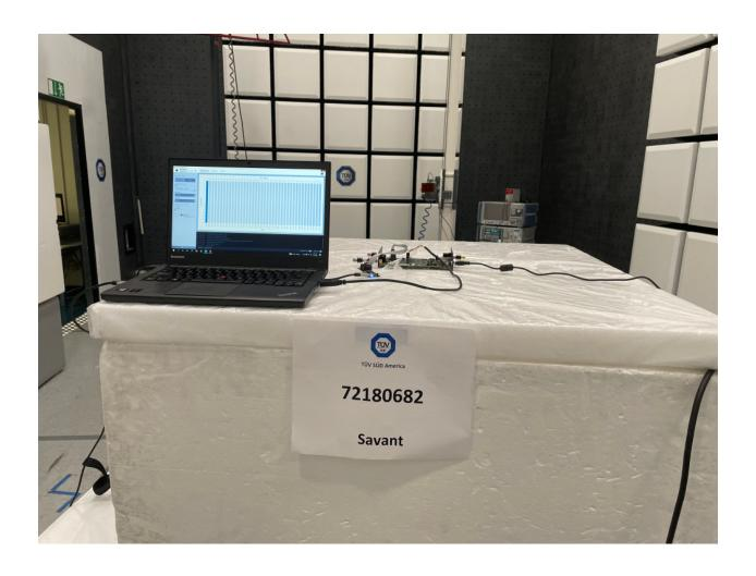
**Radiated Emissions Test Setup (Back)**
