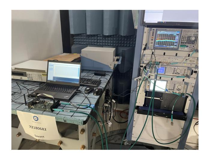
**Antenna Conducted Port Test Setup**
