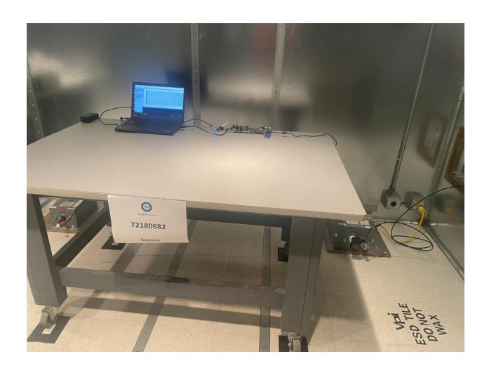
**AC Conducted Emissions Test Setup**
