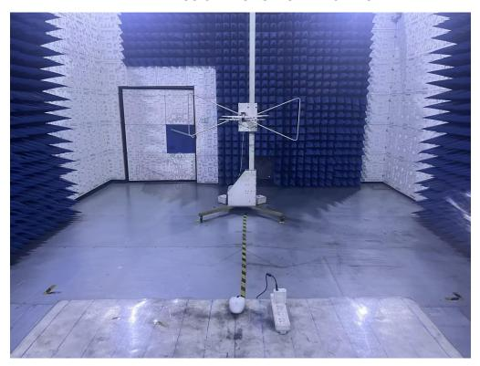
RADIATED EMISSION TEST SETUP ABOVE 1GHz
