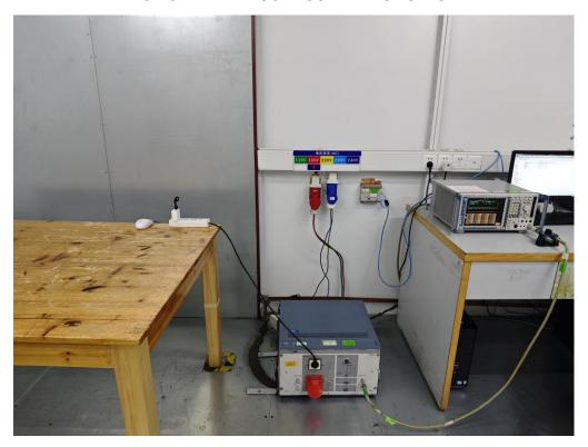
BLE RF CONDUCTED TEST SETUP
