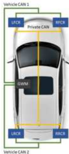
Figure 2 CubTEK 77GHz 4R Angular radar system architecture diagram
