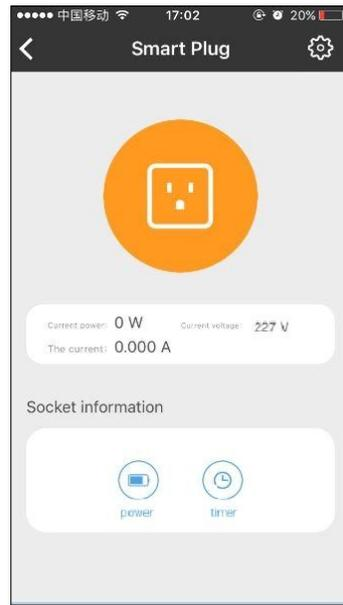
6. When in this mode, the user can view the current electricity load status, electric usage, and set the timing operation. *(Timing function is being upgraded)*
