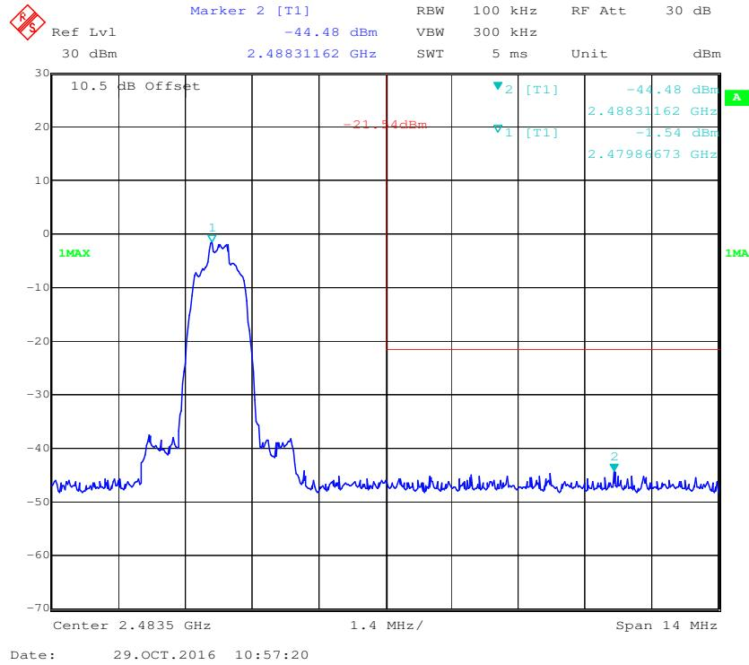
**EDR (8DPSK): Band Edge-Left Side**
