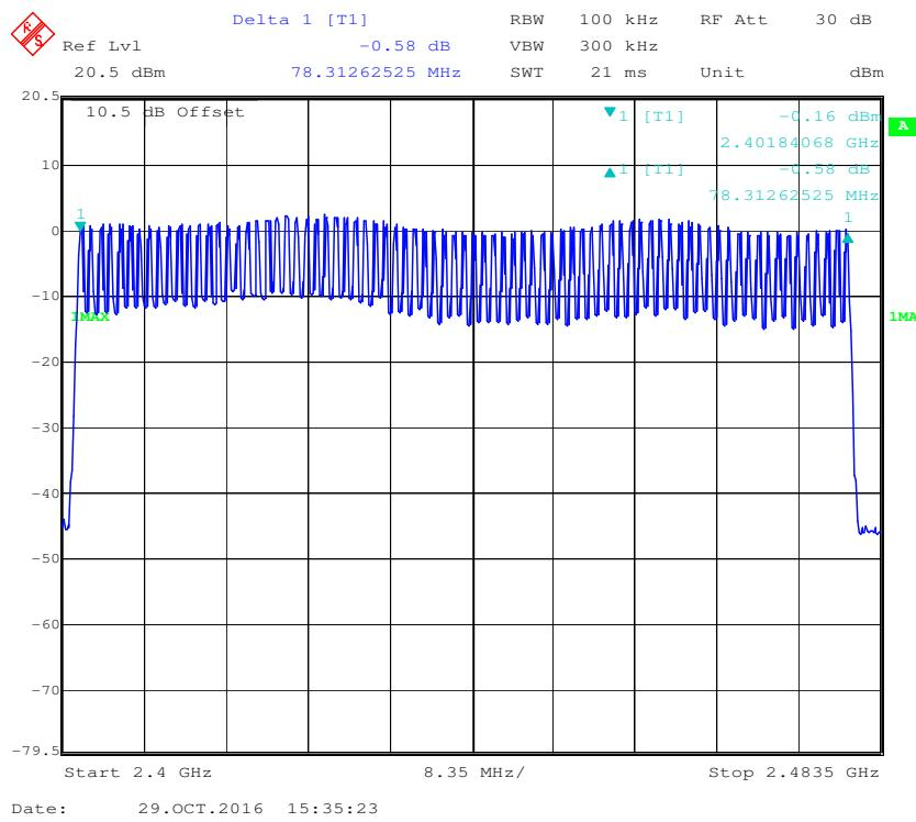
**EDR ( $\pi/4$ -DQPSK): Number of Hopping Channels**
