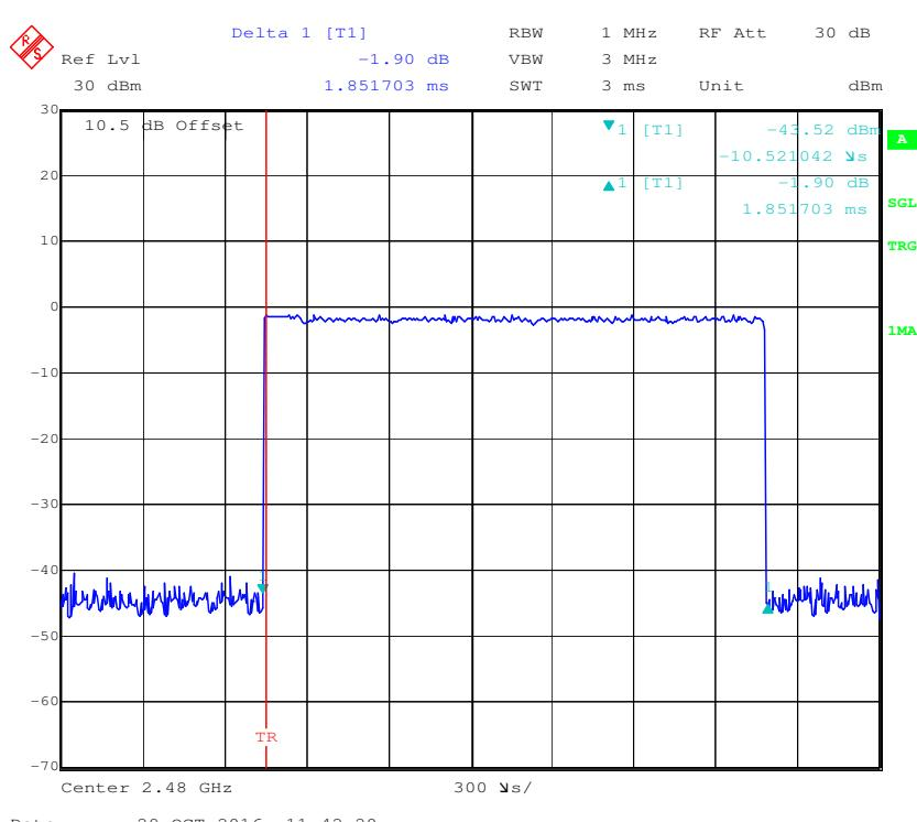
**Pulse time, Low Channel, 3DH5**
