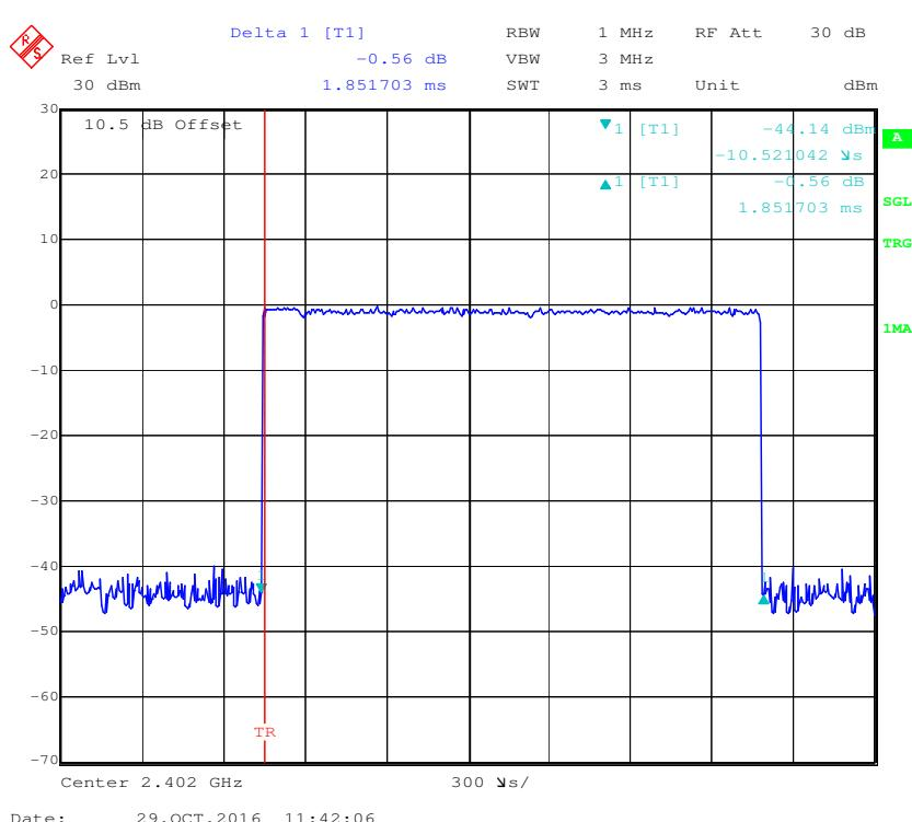
**Pulse time, Middle Channel, 3DH3**
