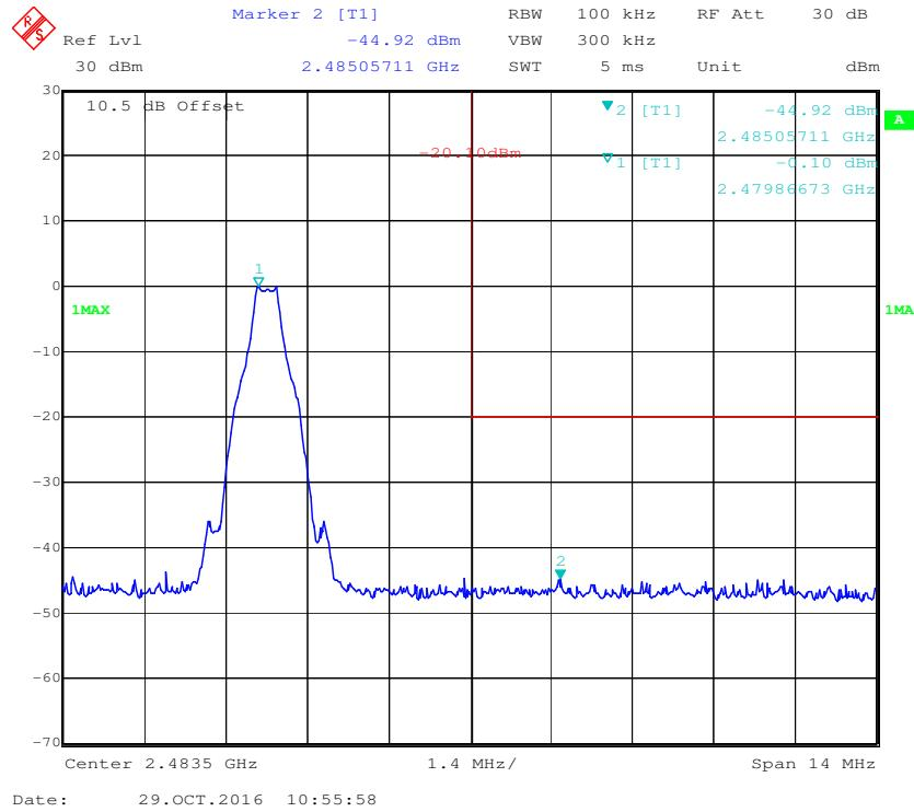
**EDR ( $\pi/4$ -DQPSK): Band Edge-Left Side**
