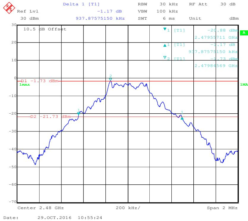
**EDR ( $\pi/4$ -DQPSK): Low Channel**
