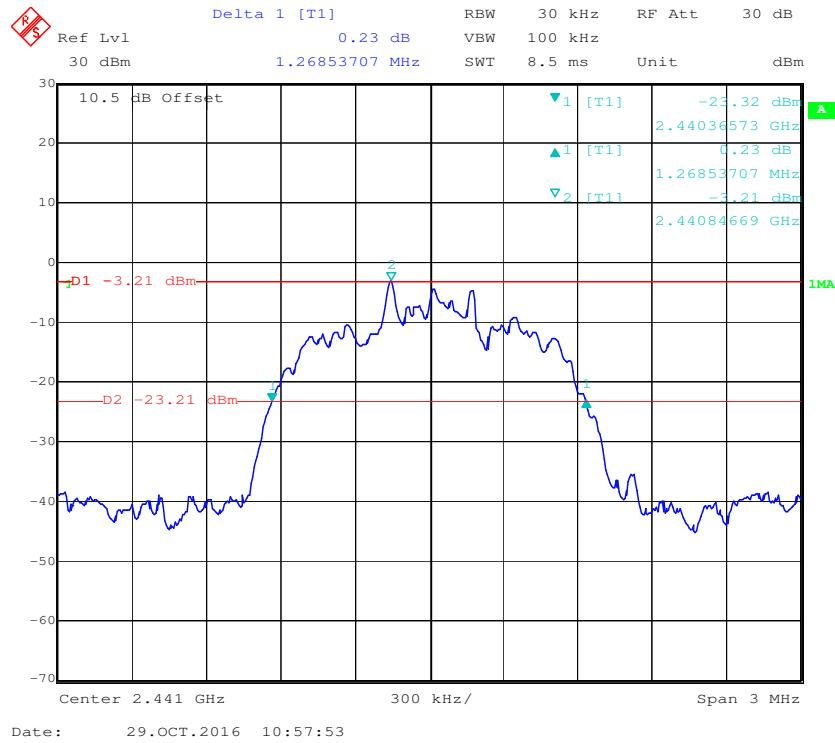
**EDR ( $\pi/4$ -DQPSK): High Channel**
