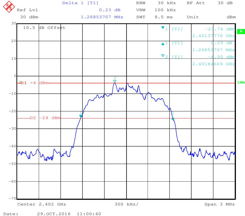
**EDR (8DPSK): Middle Channel**
