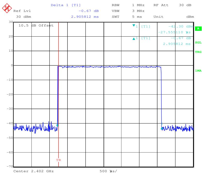
**Pulse time, Middle Channel, 2DH5**
