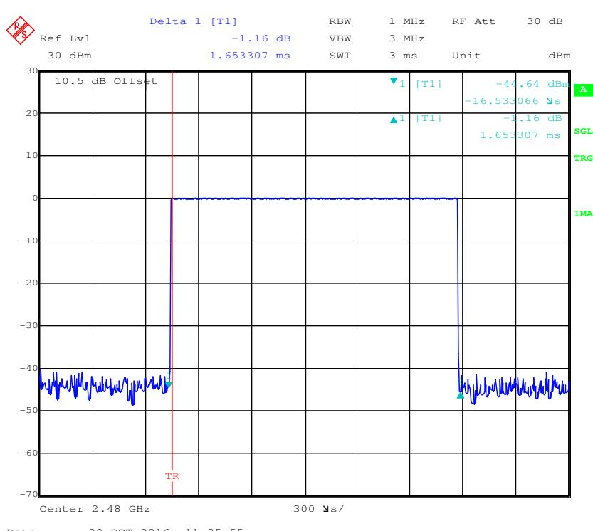
**Pulse time, Low Channel, DH5**
