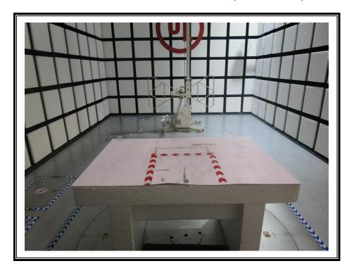
RADIATED RF MEASUREMENT SETUP (Below 30MHz)
