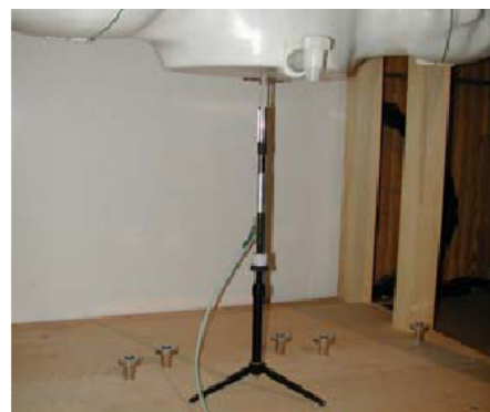
Figure 12.1 Dipole Validation Test Setup
