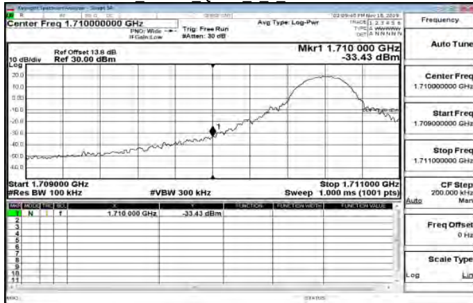
LTE\Band4 10MHz QPSK 1 49 HighCH20350-1750
