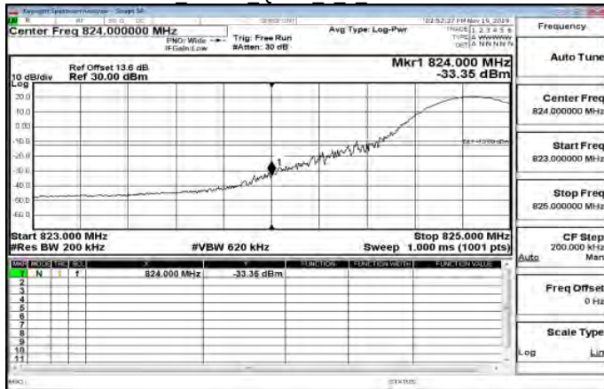
LTE\Band26 15MHz QPSK 1 0 LowCH26865-831.5
