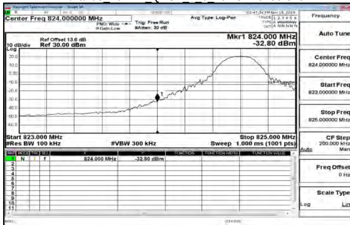
LTEBand5 10MHz QPSK 1 49 HighCH20600-844
