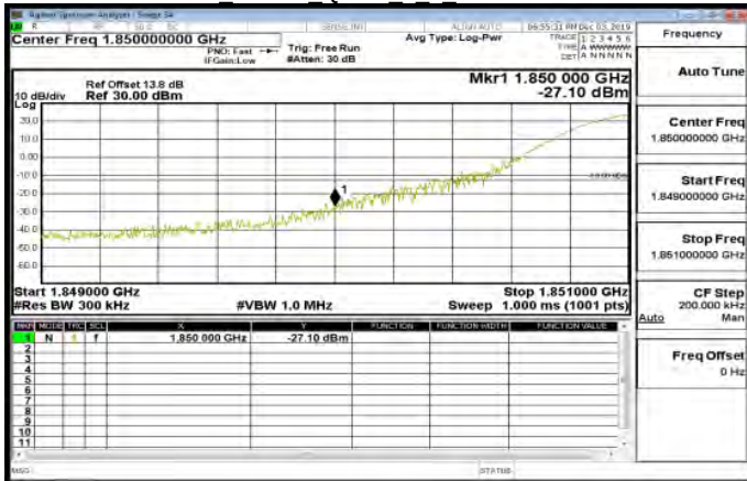
LTEBand25 20MHz QPSK 1 99 HighCH26590-1905
