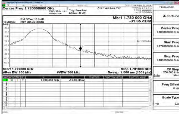
LTE\Band66 10MHz QPSK 1 49 HighCH132622-1775
