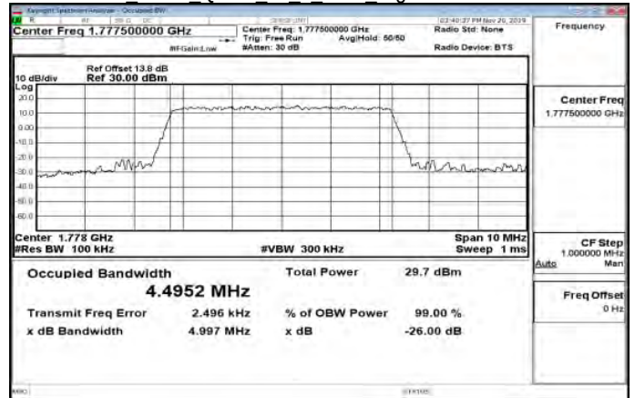
Band66 5MHz 16QAM 25 0 Main LowCH131997-1712.5
