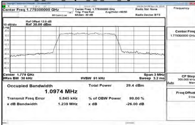
Band66 1 4MHz 64QAM 6 0 Main LowCH131979-1710.7
