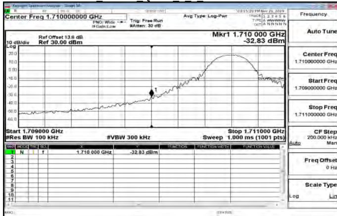
LTE\Band66 10MHz QPSK 1 49 HighCH132622-1775
