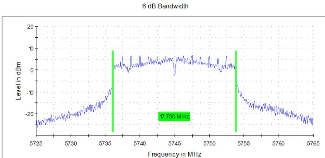
**Graph 11: Antenna 1 – 6 dB Emissions Bandwidth Transmitting at 5745 MHz - Setting 20**
