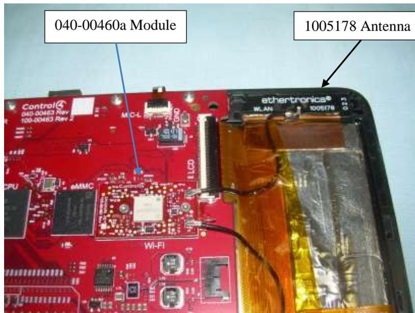
**Photograph 18: 040-00460a Installed in C4-T4T8-XX with 1005178 Antenna Installed**
