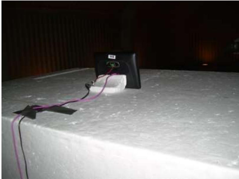
**Photograph 5: Radiated Emissions Configuration – Tabletop Unit Vertical Placement**
