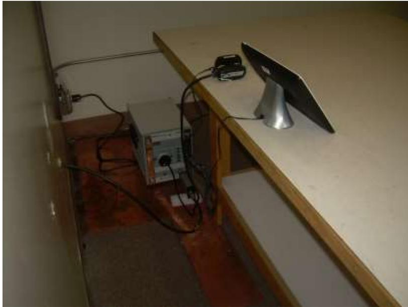
**Photograph 9 – Back View Conducted Emissions Configuration – Tabletop Units**
