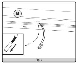
8. Connect the fixture wires to the supply wires: black to black, white to white, and green to copper/bare. **WARNING:**If there is no ground supply wire, stop installation and consult a qualified electrician.
