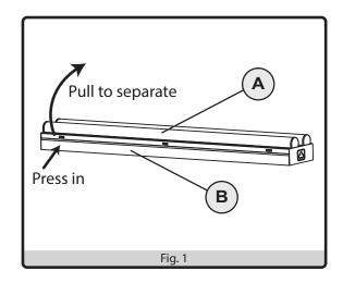
2. Locate the wiring quick disconnect connectors between the two halves and release the connectors to separate the wires between the two halves. Set aside the LED cover assembly (A). Please note to remove the screw which fixed on sensor.
