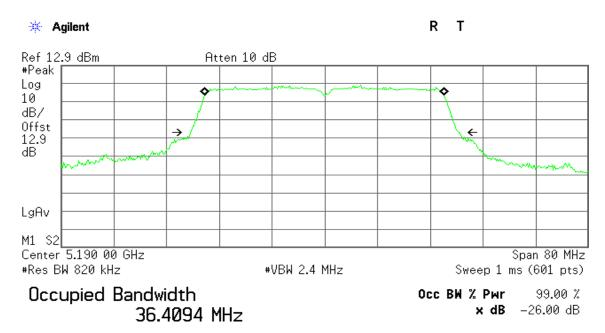
Transmit Freq Error -45.722 kHz x dB Bandwidth 40.751 MHz
