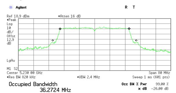
Transmit Freq Error -56.247 kHz x dB Bandwidth 40.251 MHz
