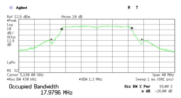
Transmit Freq Error -18.289 kHz x dB Bandwidth 21.363 MHz
