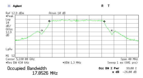
Transmit Freq Error -4.380 kHz x dB Bandwidth 20.855 MHz
