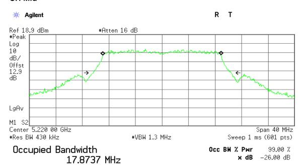
Transmit Freq Error -9.906 kHz x dB Bandwidth 20.849 MHz
