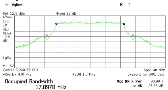
Transmit Freq Error 3.573 kHz x dB Bandwidth 20.994 MHz
