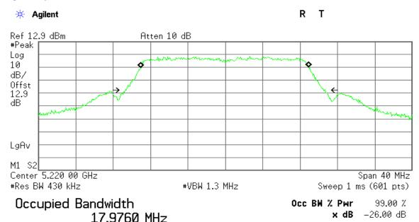
Transmit Freq Error -52.556 kHz x dB Bandwidth 21.377 MHz
