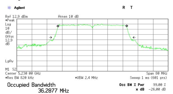
Transmit Freg Error -63.798 kHz x dB Bandwidth 40.137 MHz
