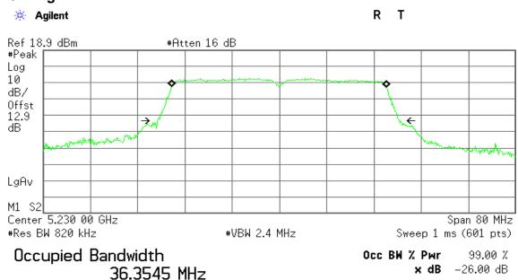
Transmit Freq Error -78.516 kHz x dB Bandwidth 40.938 MHz
