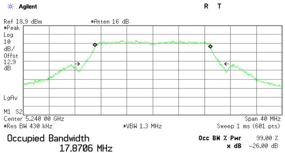
Transmit Freq Error -15.430 kHz x dB Bandwidth 20.982 MHz
