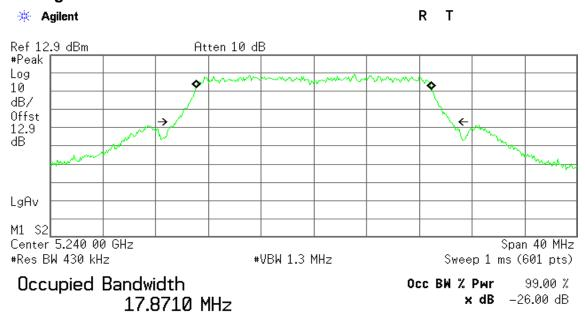
Transmit Freq Error -4.630 kHz x dB Bandwidth 20.783 MHz
