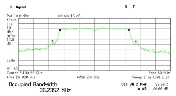
Transmit Freq Error -19.864 kHz x dB Bandwidth 40.155 MHz
