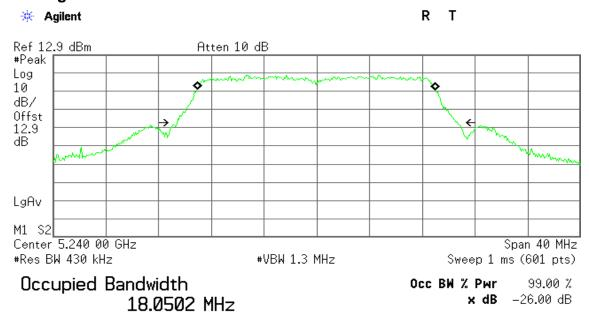
Transmit Freq Error -48.196 kHz x dB Bandwidth 21.279 MHz
