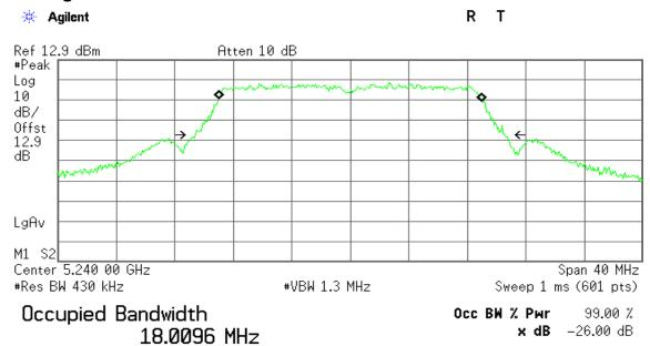
Transmit Freq Error -1.427 kHz x dB Bandwidth 21.205 MHz
