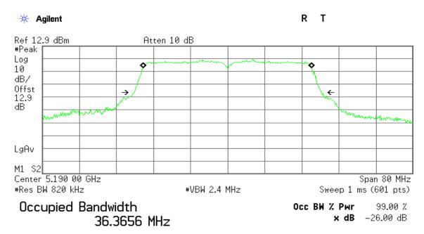
Transmit Freq Error -53.215 kHz x dB Bandwidth 40.390 MHz
