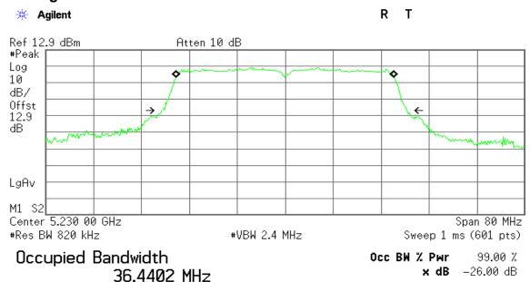
Transmit Freq Error -21.533 kHz x dB Bandwidth 40.832 MHz
