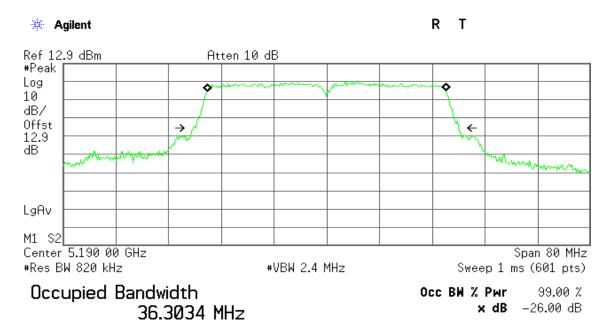
Transmit Freq Error -34.447 kHz x dB Bandwidth 40.352 MHz
