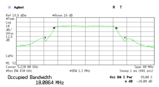
Transmit Freq Error -36.030 kHz x dB Bandwidth 21.380 MHz
