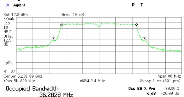
Transmit Freq Error -39.627 kHz x dB Bandwidth 40.235 MHz
