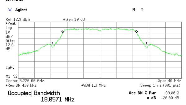
Transmit Freq Error -28.530 kHz x dB Bandwidth 21.322 MHz
