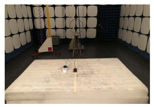
3. Radiated emission (9KHz-30MHz)
