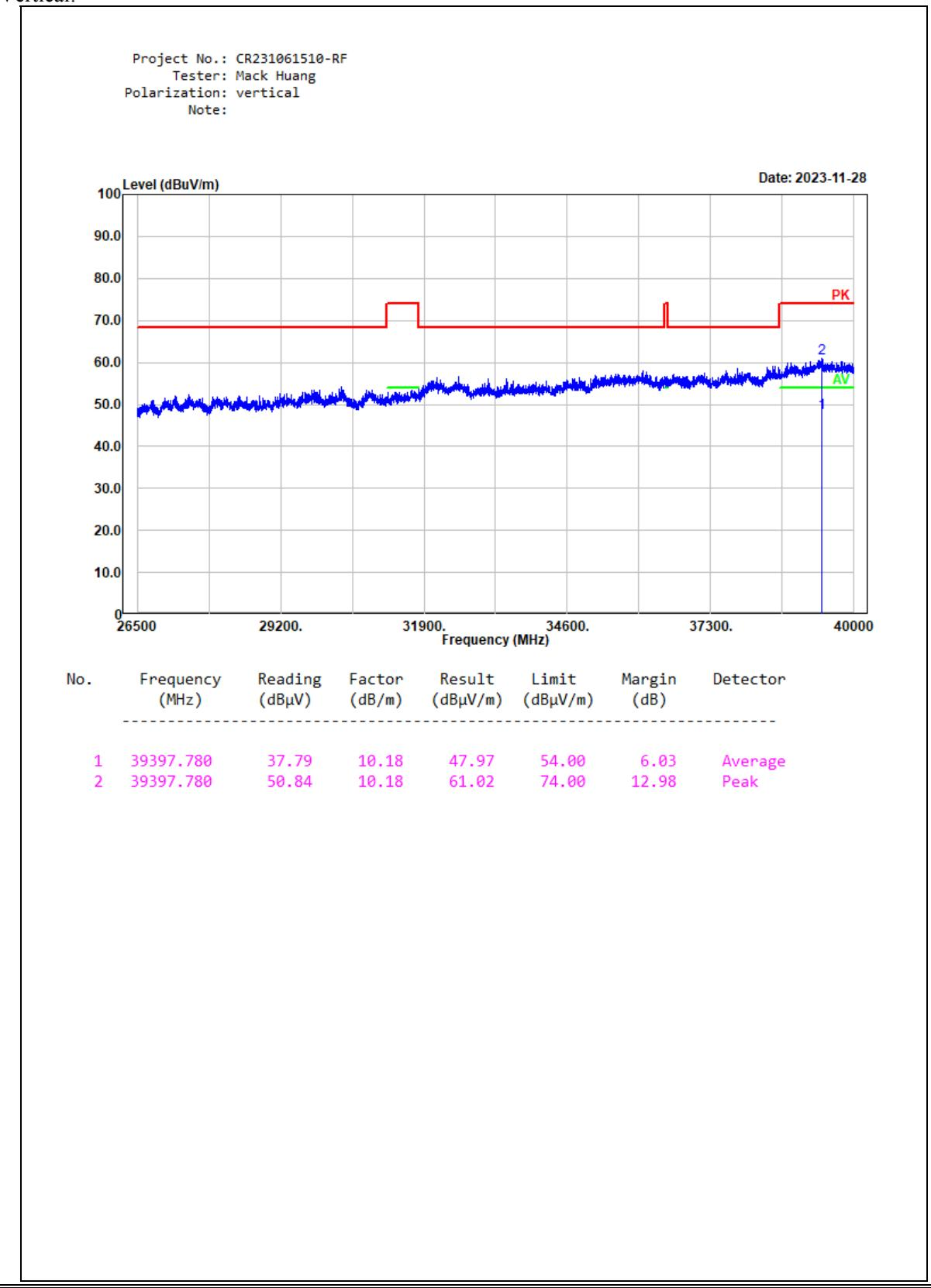
**Band Edge Measurements (Radiated):**
