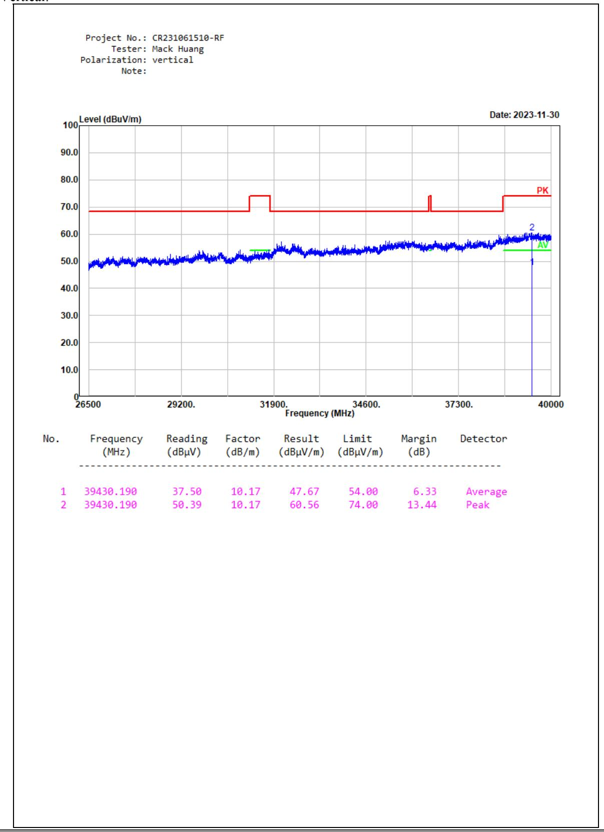
**Band Edge Measurements (Radiated):**
