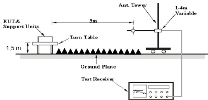
The radiated emission tests were performed in the 3 meters chamber test site, using the setup accordance with the ANSI C63.10-2013. The specification used was FCC 15.209, FCC 15.407 limits.
