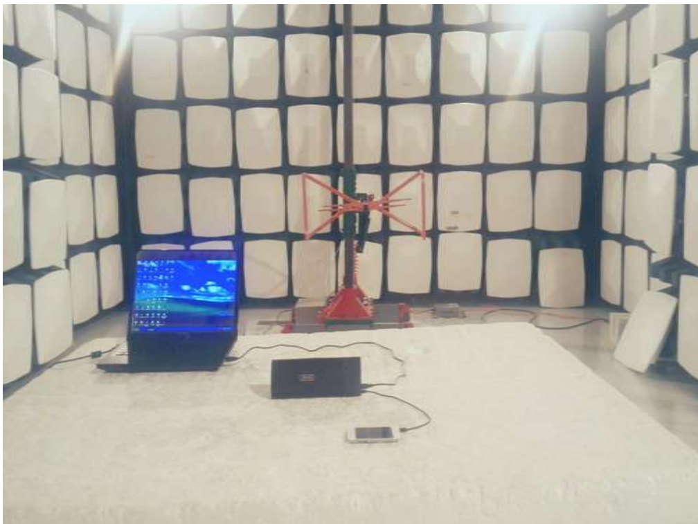
FCC RADIATED EMISSION TEST SETUP
