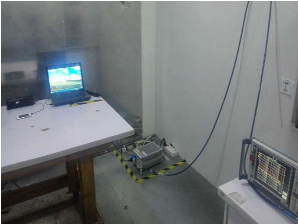
FCC RADIATED EMISSION TEST SETUP
