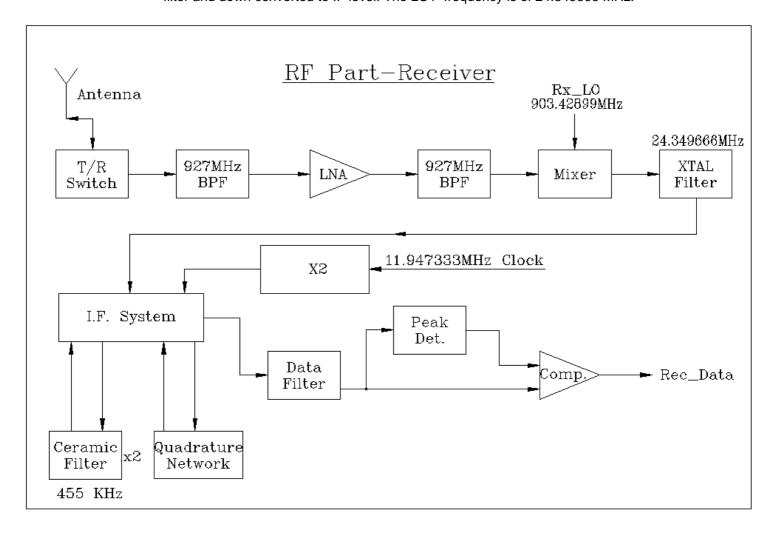
The IF signal enter to crystal filter (BPF) and entered to standard FM discriminator integrated circuit. The output of the discriminator enters to threshold comperator that generates the data signal.
