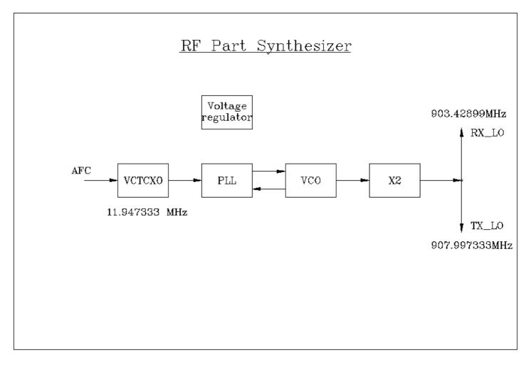
The clock sourse based on a standard VCTCXO controlled by the CPU. The compensation value is calculated and it is using to control the VCTCXO.
