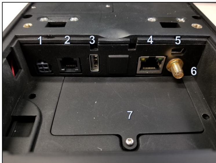
Figure 2: ACR330 Connection Ports
