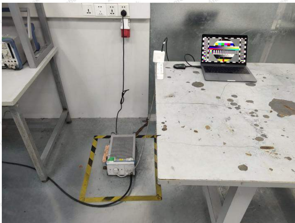
Photo of Power Line Conducted Emission Test
