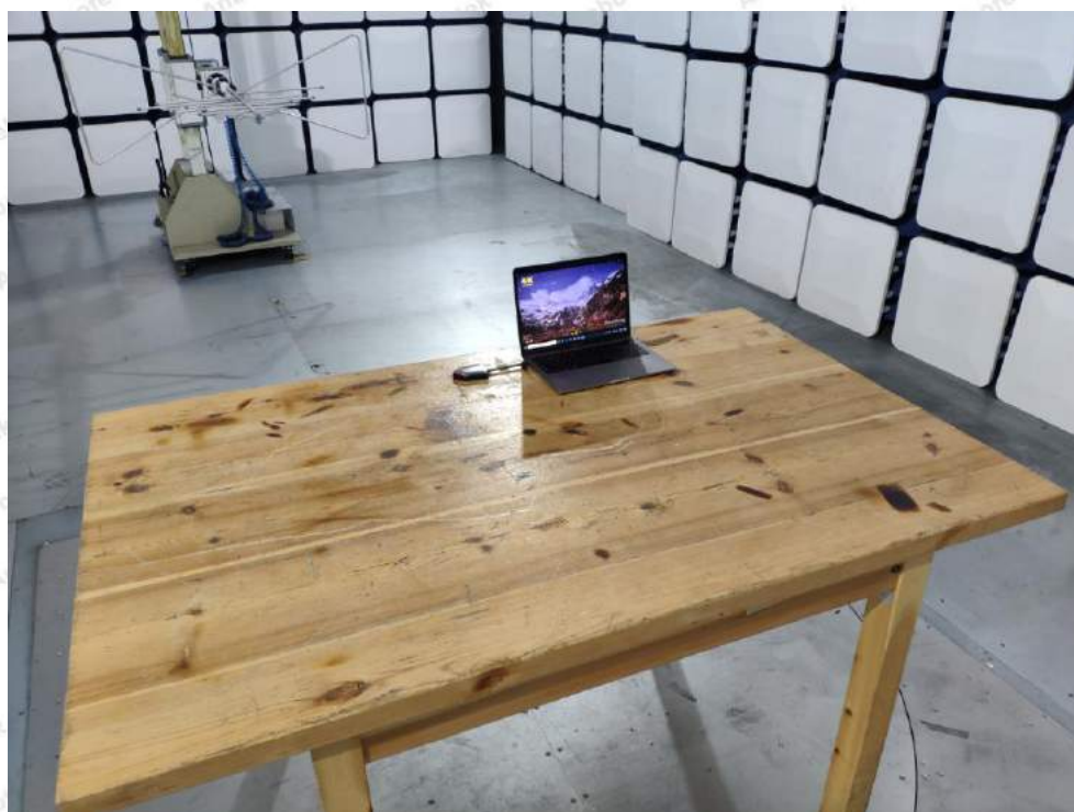
Photo of Radiation Emission Test
