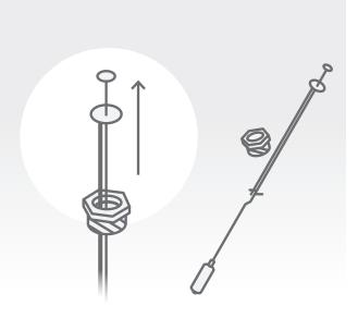
**e.** Remove the steel wire assembly from the bushing by gently pulling it upward while holding the bushing.
