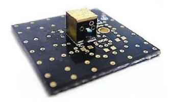
Compliance with FCC 15.203 is achieved as the antenna is permanently fixed inside our Bluetooth device and is soldered to the printed circuit board. To replace the antenna, the case of the device must be broken, and the solder removed.
