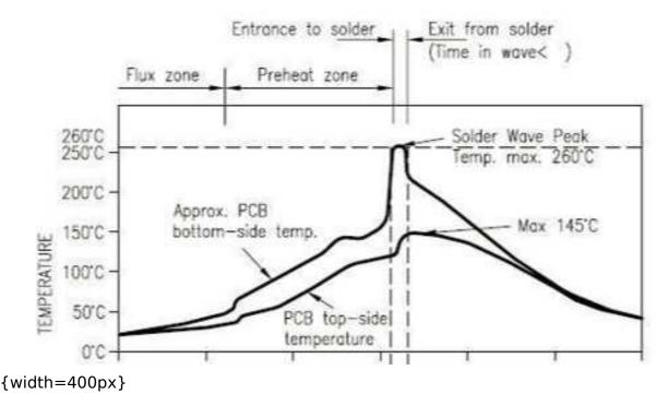
Recommended soldering temperature:
