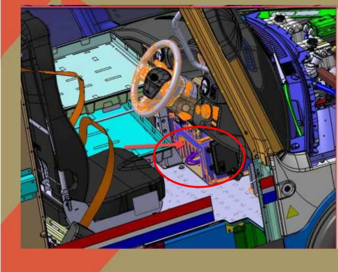
The TCU is mounted in a module box which is installed at the bottom of the center console of the vehicle.
