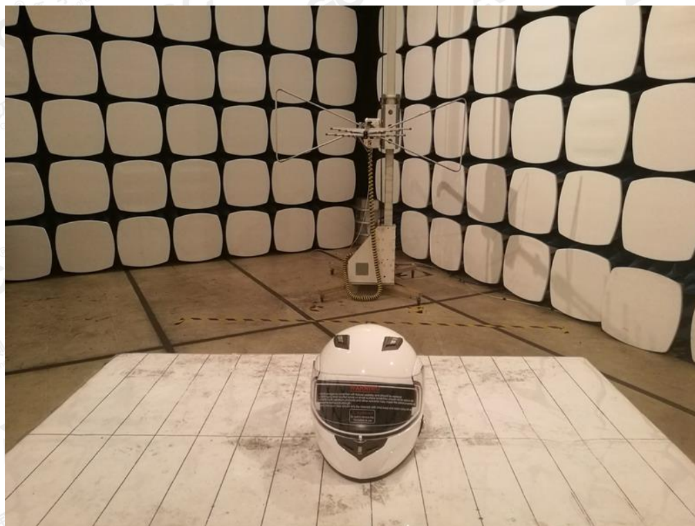
FCC RADIATED EMISSION TEST SETUP
