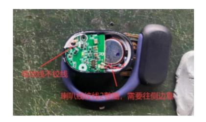
As shown in the figure, the battery line is not twisted, the horn wire is twisted 2 whole circle, and leans to the outside.
