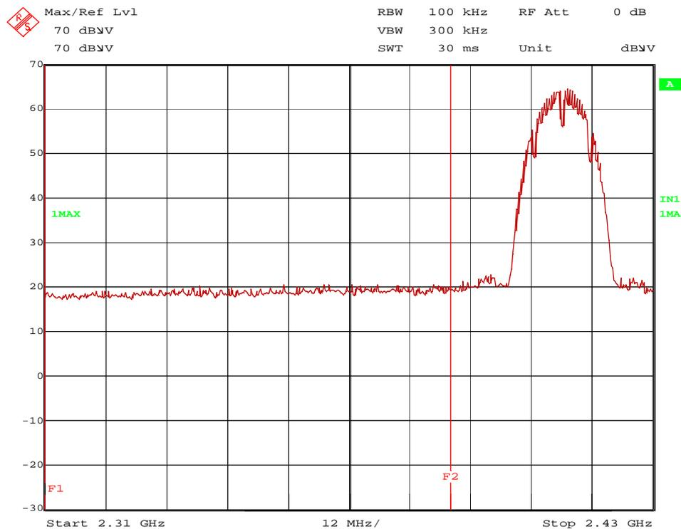
145298 #23 bandedge restr ch11 1Mbps.wmf: radiated band-edge compliance (operation mode 3):
