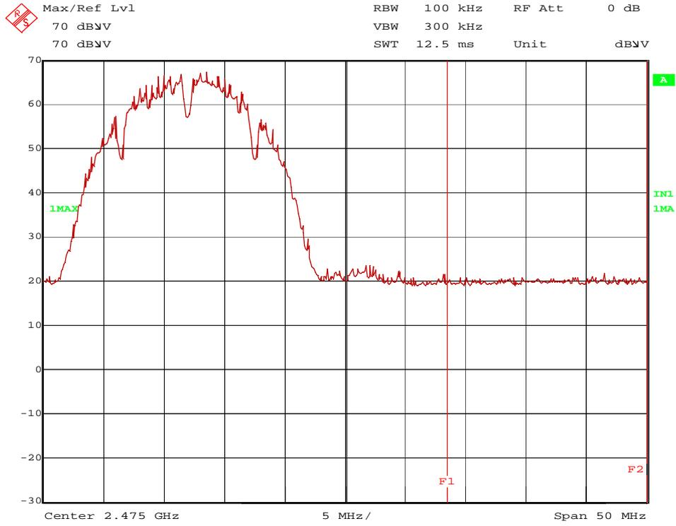
145298 #23 bandedge restr ch11 6Mbps.wmf: radiated band-edge compliance (operation mode 7):
