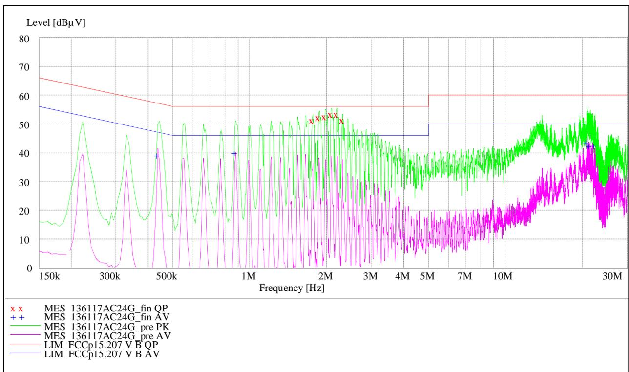
Result measured with the quasipeak detector (marked by an x):
