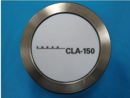
The Loop Antenna used is based on the IEEE-1528 standard, the table below provides details for the mechanical and electrical Specifications for the Loop Antenna.
