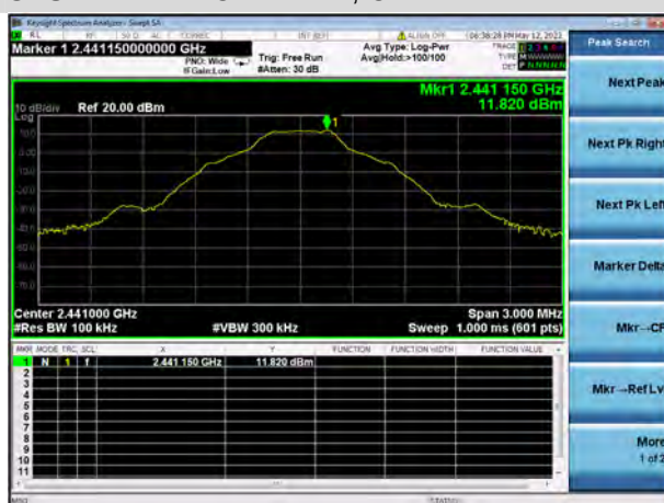
GFSK MIDDLE CHANNEL, CARRIER LEVEL
