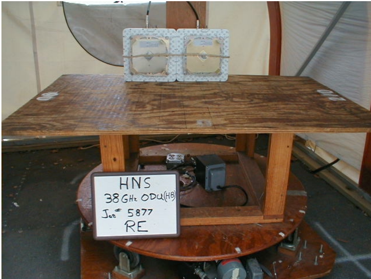
Figure 36 Test setup photo1 for Radiated Spurious Emission in open field site for Both Hub and Sub 38 GHz High band ODUs (30 Mhz- 18 Ghz)
