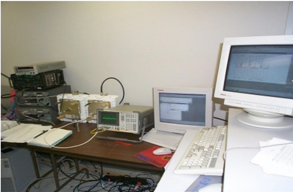
Figure 23 Test setup photo2 for Conducted Spurious Emission for Both Hub and Sub 38 GHz High band ODU.
