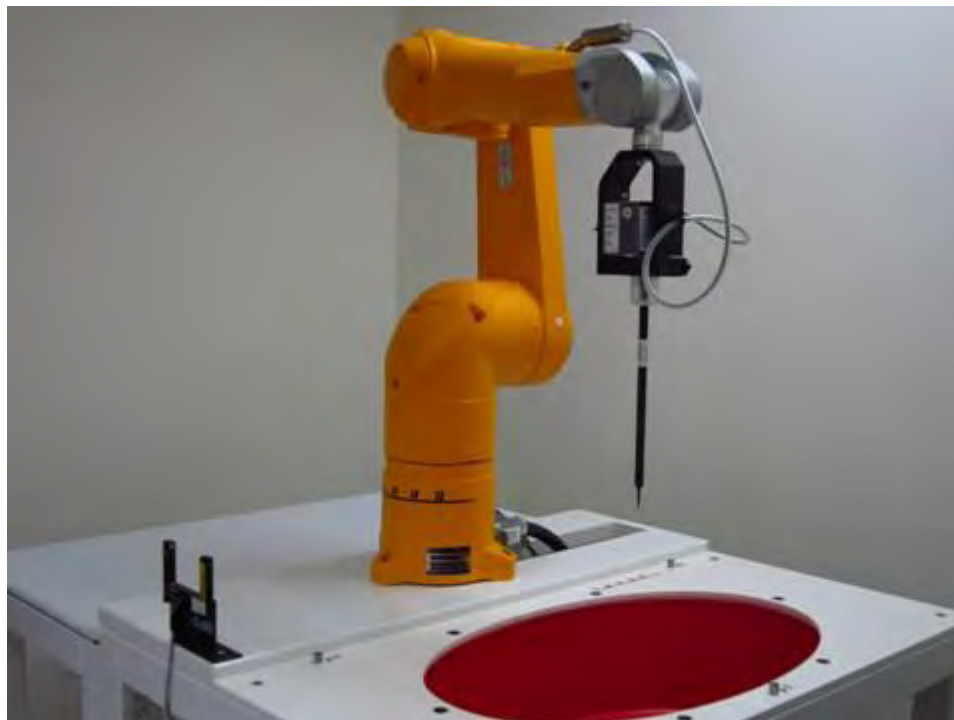
Fig.1 Photograph of the SAR measurement system
