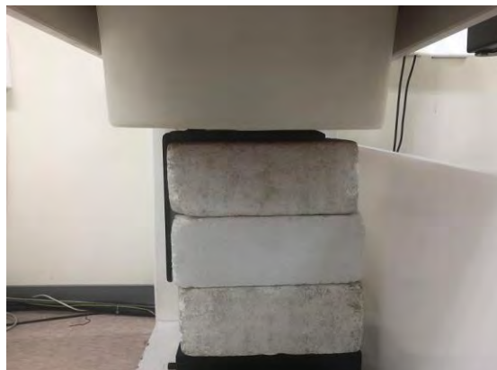
Fig.3 EUT Bottom side to flat phantom
