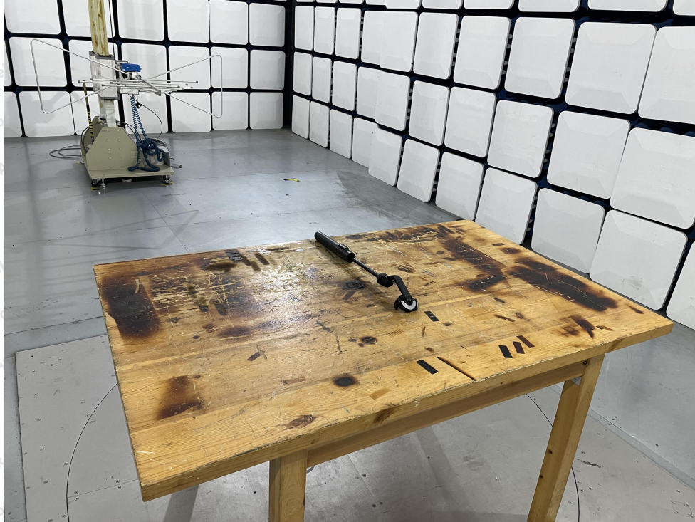
Photo of Radiation Emission Test (below 1GHz)
