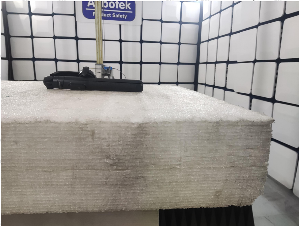
Photo of Radiation Emission Test (above 1GHz)
