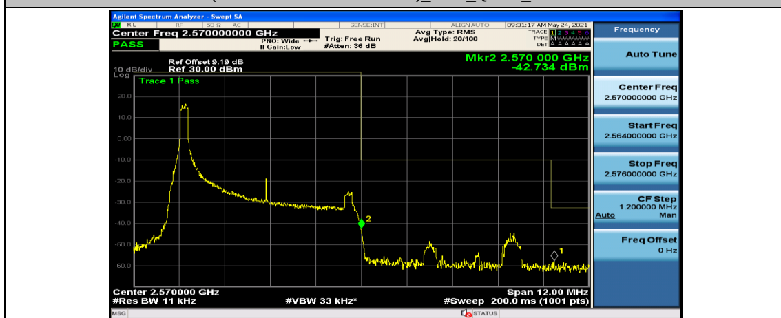
(Channel Bandwidth: 5 MHz)_HCH_QPSK_1RB#12
