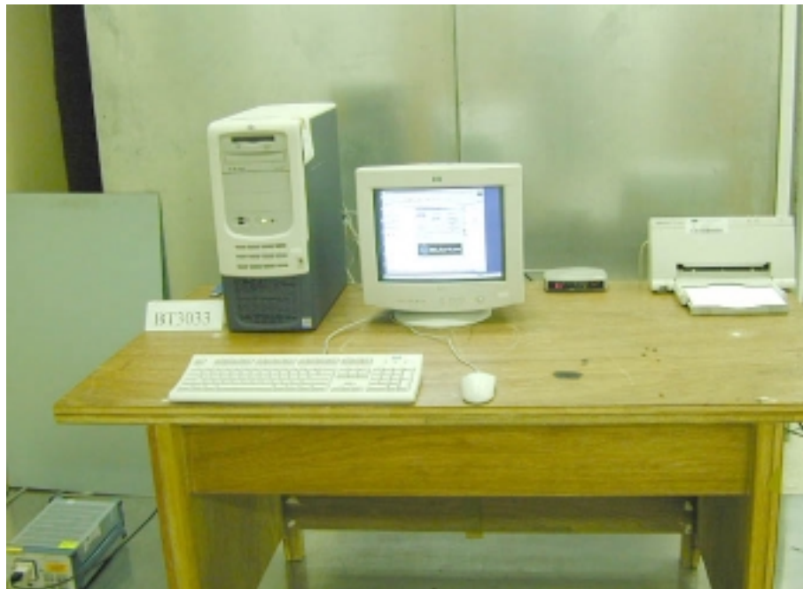
Photo 1: Conducted Test Set-up (front)
