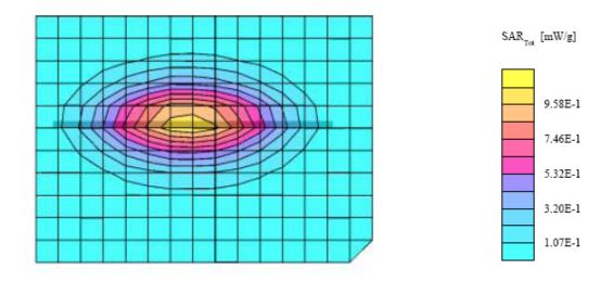
System Validation 835 MHz Head liquid (Ambient Temp = 23 Deg C, Liquid Temp = 22 Deg
