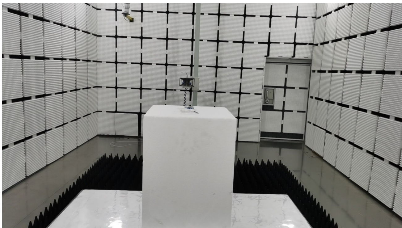
Photograph 2: Set-up for Radiated Spurious Emission, Above 1GHz
